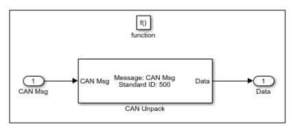
The reason to place the CAN Unpack inside a Function-Call Subsystem is so that it can capture all possible messages.
