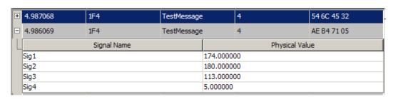
The tool displays the signal name as defined in the attached database and the signal's physical value.
